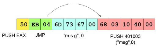
In this example, a linear disassembler would try to disassemble bytes 6D 73 67... as an instruction instead of interpreting it as text string. Resulting disassembly would look as follows:
