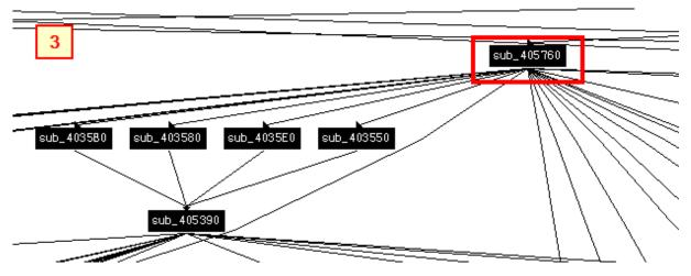
If you look closer at the rest of the graph you notice several other potentially interesting functions like *sub\_4027E0* performing some file system operations (*DeleteFileW, WriteFile, SetFileAttributesW, CreateFileW*) or *sub\_406CA0* doing some threads operations (*ResumeThread, SuspendThread, OpenThread, ...*).
