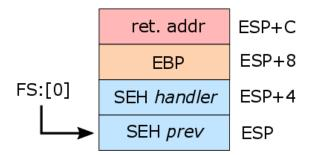
The next question should be whether any exception is triggered in this function? Yes, take a look at the *ecx* register: First, it is zeroed and then the program tries to write a DWORD value to the address pointed by this register. However, because *ecx* points to unallocated address *0x00000000* this will cause an exception (STATUS\_ACCESS\_VIOLATION – 0xC0000005) and program execution would be switched to the installed exception handler.
