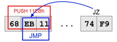
As you see the hidden jump is again leading us into the middle of an instruction at *0x40105D* (to the address *0x40105E*). But this time it looks like a normal assembly desynchronization.
