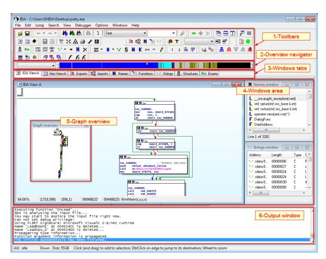
The central part of the workspace is occupied by the *Windows area* (4). IDA uses multiple windows to present various types of information about the disassembled binary. Among the most frequently used windows are:
