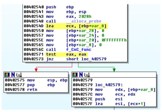
You are now at the beginning of the *sub\_402540*. It seems there are no push instructions before a call to *f\_CnC\_func*. However notice that *ecx* register is assigned with the address of *var\_8* variable, which is later also initialized to zero.
