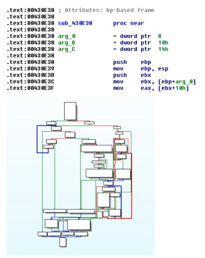
Unfortunately, this won't always work – especially if malware is using anti-disassembly techniques. In such case you may do analysis using only text view mode or try to correct code manually.
