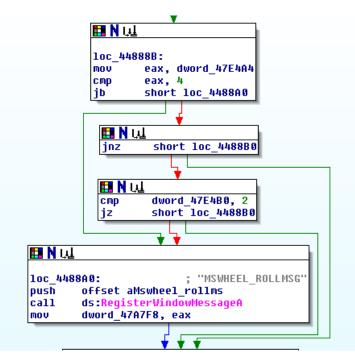
Different colours of the lines are used to indicate different types of code transitions:
