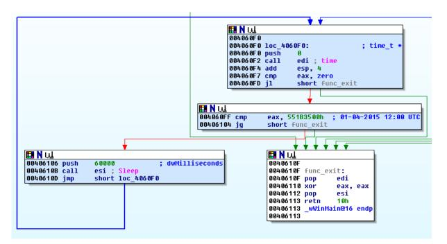
The next three blocks, create a loop. All the loop does is to check system time and compare it to previously checked date of 01 April 2015. If time is greater than this date, the program quits. Otherwise, the program sleeps one minute (60,000 milliseconds) and repeats checking the date.
