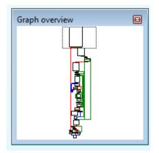
If the function graph is too big to fit your current disassembly view size, your current position will be marked with a small dotted rectangle within the *Graph overview* window. This rectangle will change size whenever you zoom in or out of the function graph.
