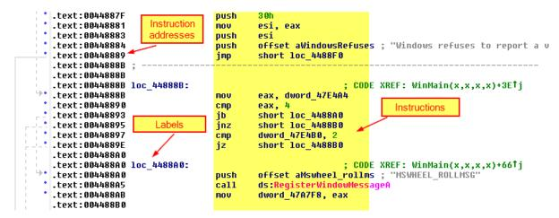
Notice the dashed and solid lines on the left side of the text view. They are used to indicate conditional and unconditional jumps, respectively. If you click on jump destination, IDA will highlight destination label as well as a corresponding arrow.
