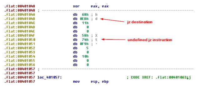
Now select the byte at *0x40104B* and press <C> to define code. Do the same with the byte at *0x401050* (*jz* instruction). After this, you should see code similar to this one:
