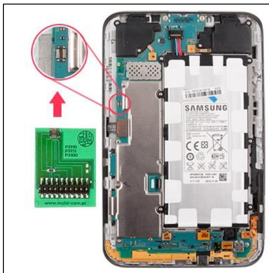
Figure 26: A JTAG connector. Source: [http://multi-com.eu/multicom/pimg/jtag\\_p3100\\_400.jpg](http://multi-com.eu/multicom/pimg/jtag_p3100_400.jpg)
