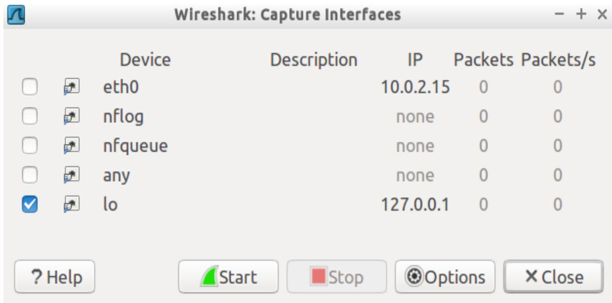
Figure 8: Selecting interface in Wireshark
