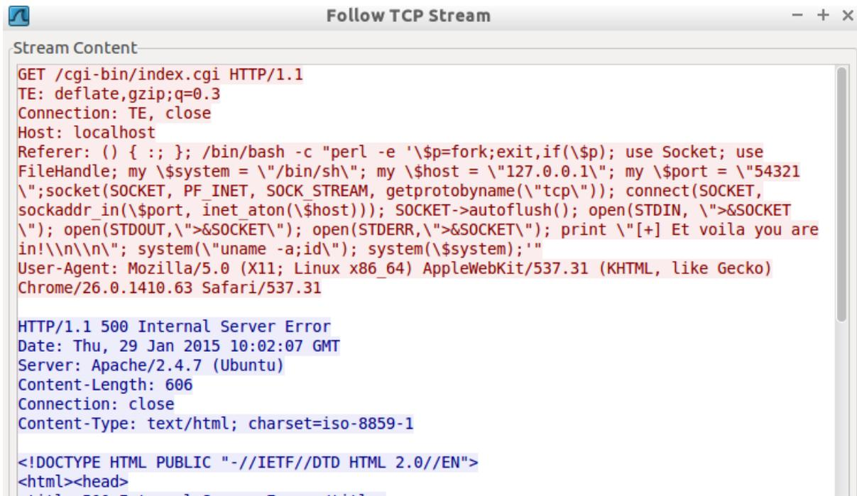
Figure 16: Following TCP stream in Wireshark.
