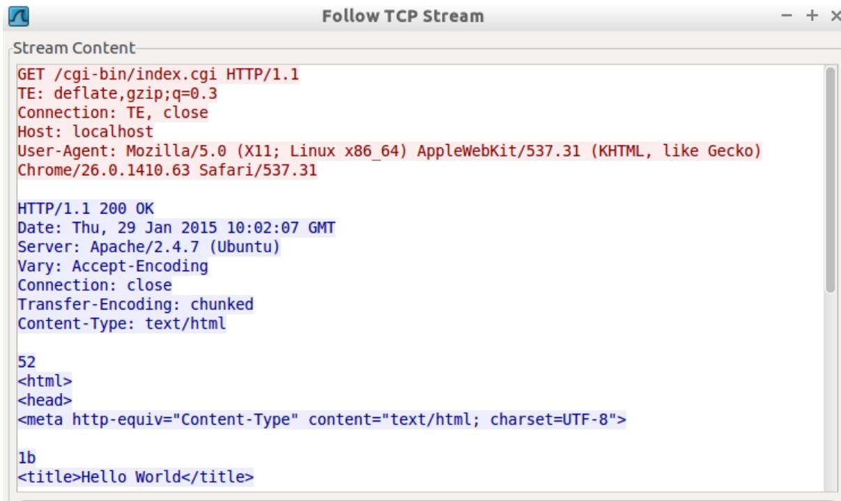
Figure 15: Following TCP stream in Wireshark.
