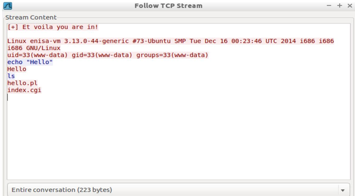
Figure 18: Following TCP stream in Wireshark.
