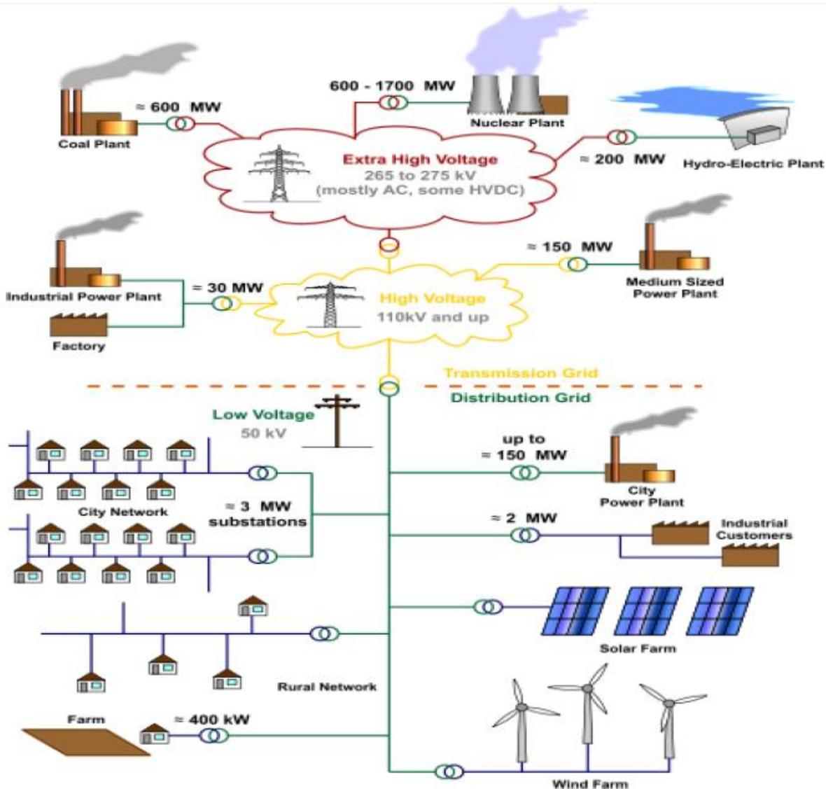
Figure 2: Grid overview map [https://en.wikipedia.org/wiki/File:Electricity\\_Grid\\_Schematic\\_English.svg](https://en.wikipedia.org/wiki/File:Electricity_Grid_Schematic_English.svg)
