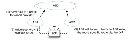
(b) **Prefix splitting.** BGP will prefer a more specific route towards a destination. By splitting up a provider's network into smaller chunks, these alternative routes will be preferred by other ASes.
