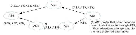
(a) **AS path padding.** BGP routing will provide a shorter path, however paths can be made artificially made longer by inserting one's own AS number into the advertised path.
