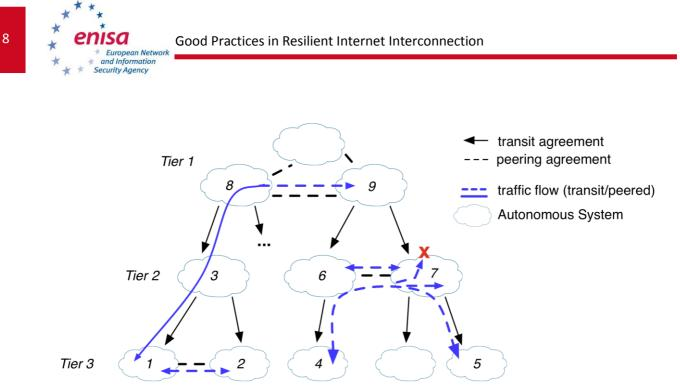
**Figure 3:** Schematic structure of the interconnection types between autonomous systems and resulting traffic flows.
