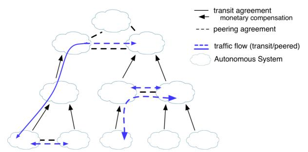
Figure 1: Network operators seek to enhance the overall areas they can provide service to by creating interconnections with other networks, usually referred to as autonomous systems (AS). These relationships are either monetary (transit) or reciprocal (peering).
