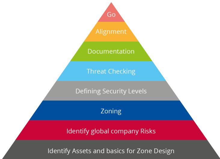
The overall process steps to define zones from scratch based on the standard processes in CLC/TS50701:2021 and EN62443-3-2:2018 are shown below. In this paper, some states are split for easier explanation.
