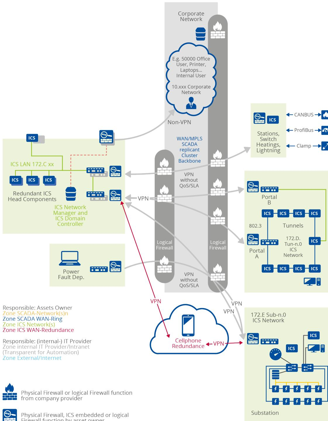
Note: the security gateways must fulfil, on both sides, the same SL and the communication must be encrypted for SL1 or higher.
