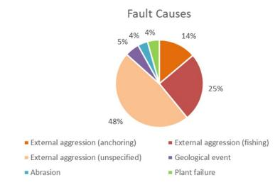
From Figure 5, one can conclude that almost 40% of cable faults are due to anchoring or fishing, whereas for almost half of them the cause is unspecified. In total, 87% of incidents are caused by human intervention, either unintentional errors or intentional malicious actions. Only 4 % of incidents are attributed to system failures (plant failures) and 5 % are due to natural phenomena.
