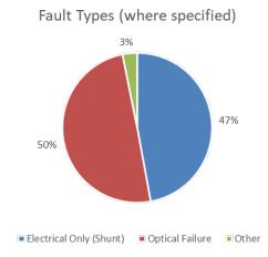
Figure 6, from the same report, shows that cable faults are evenly split between faults of the electrical system (shunt failures) and the optical system (fibre failures).
