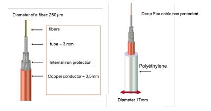
From right to left <sup>72</sup>, from no armour (for the deep sea) to double armoured (for shallow waters).
