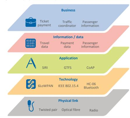
Figure 9 Data exchange from the perspective of an IPT operator
