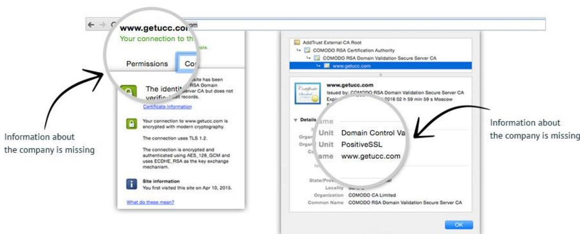
Figure 4: Example of a DV certificate<sup>11</sup>
