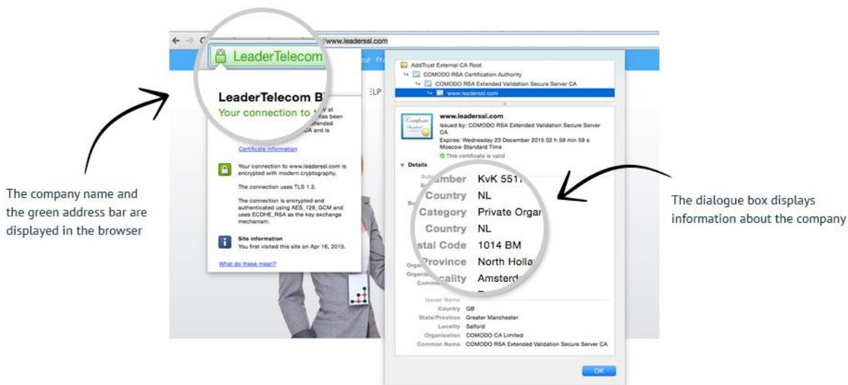
Figure 6: Example of an EV certificate<sup>12</sup>
