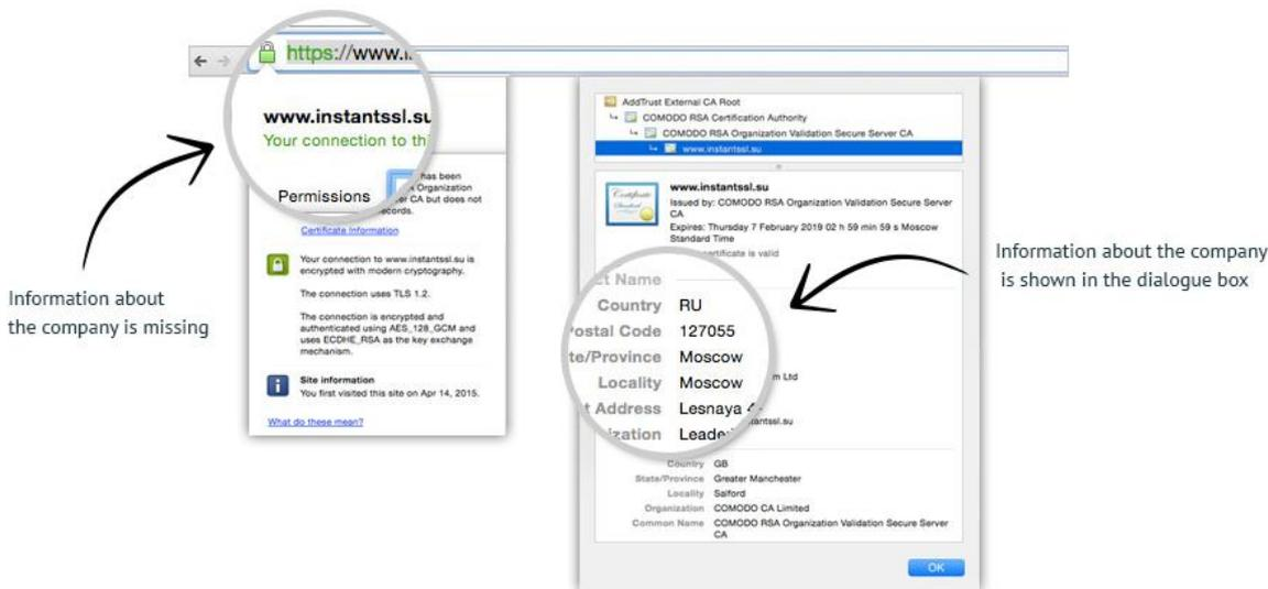
Figure 5: Example of an OV certificate<sup>12</sup>
