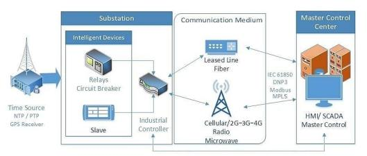
Figure 1: Functional architecture of time-phase data processing on the power grid
