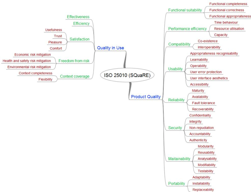
**Figure 4. ISO 25010 – Systems and Software Quality Requirements and Evaluation (SQuaRE).**
