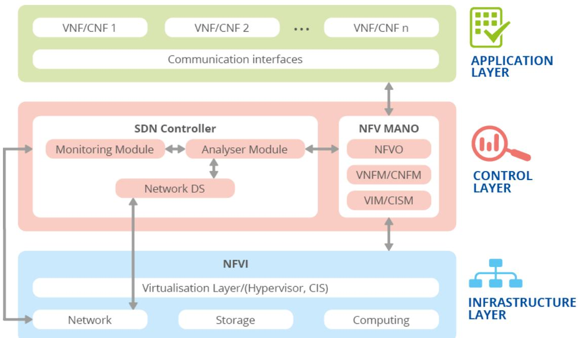
The SDN controller centralises the control plane functionalities and provides an abstract view of all the connectivity-related components it manages. The SDN Controller sets up and manages the underlying networking resources to provide the required connectivity for communicating the VNFs. Managed by the VIM, this controller may change infrastructure behaviour on-demand according to VIM specifications, adapted from the requests of tenants.
