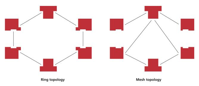
In the backbone typically ring or mesh topology is applied (Figure 7).
