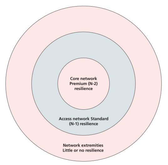
Figure 12: Resilience levels shown increasing towards the network core
