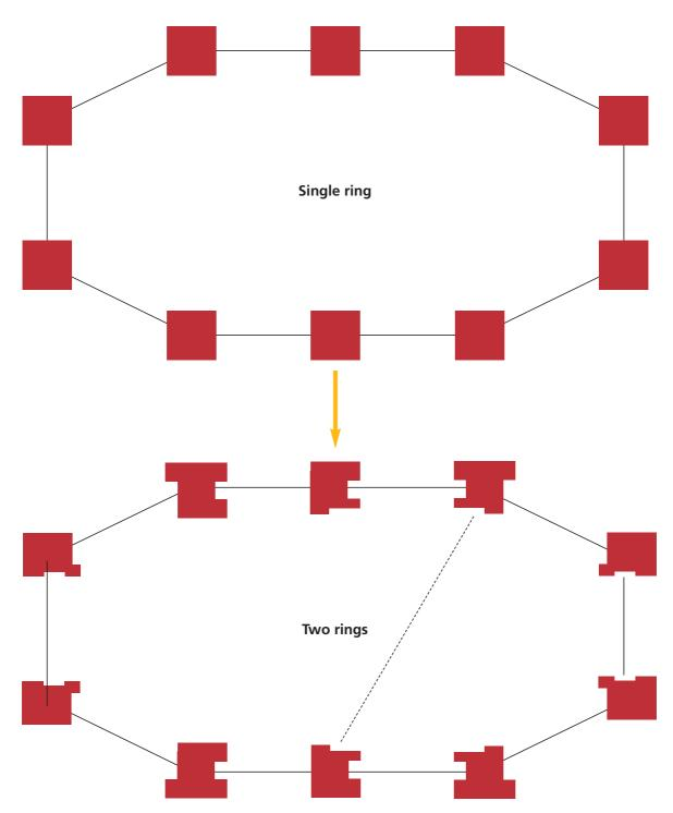
Figure 8: Example of extension of the single ring into a multi-ring topology
