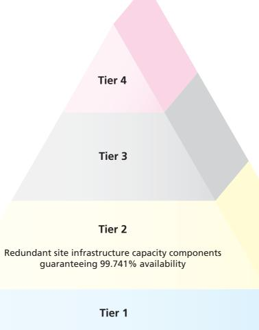
Single non-redundant distribution path serving the IT equipment Non-redundant capacity components Basic site infrastructure guaranteeing 99.671% availability NOTE: Each succeeding tier encapsulates the requirements of the preceding tier
