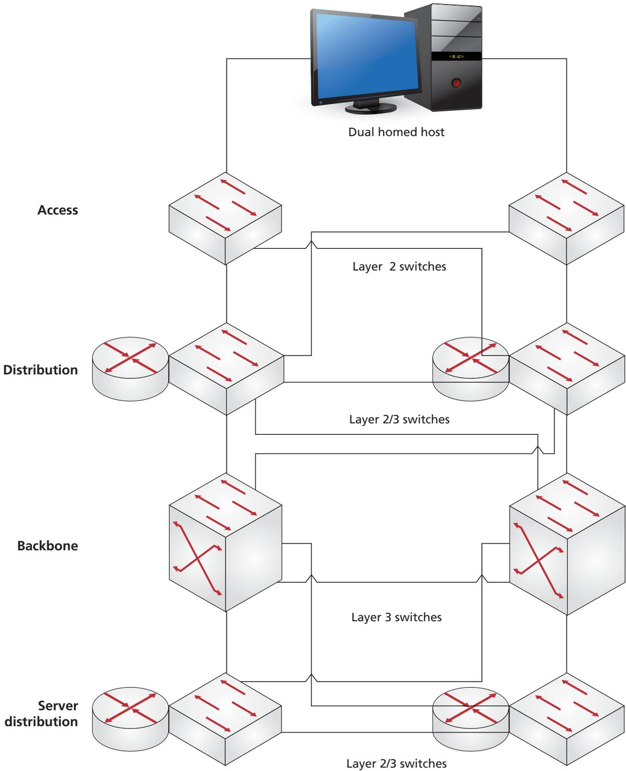
Figure 6: Redundant network with no single points of failure
