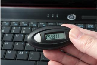
Figure 3 Hardware Token (time based OTP).
