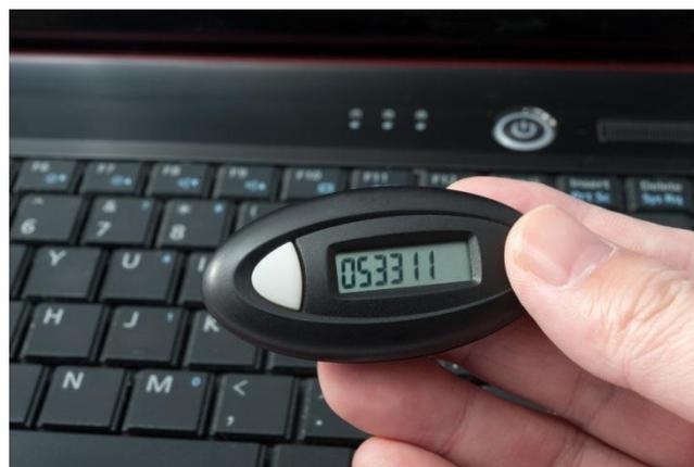
Figure 3 Hardware Token (time based OTP).
