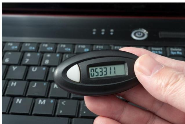
Figure 3 Hardware Token (time based OTP).
