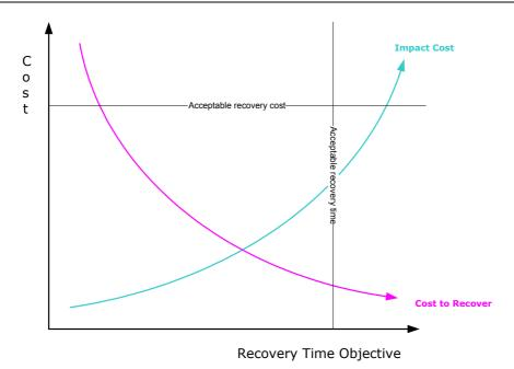
Figure 18 - Recovery cost vs RTO.7
