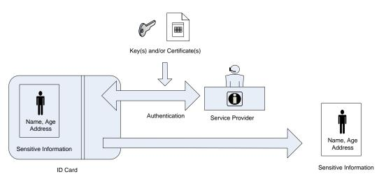
Figure 3: Access Control: Authentication of Service Provider
