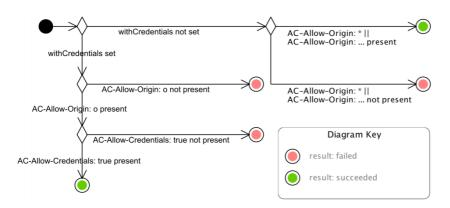
The sub-diagram below shows the resource sharing check from the main activity diagram.
