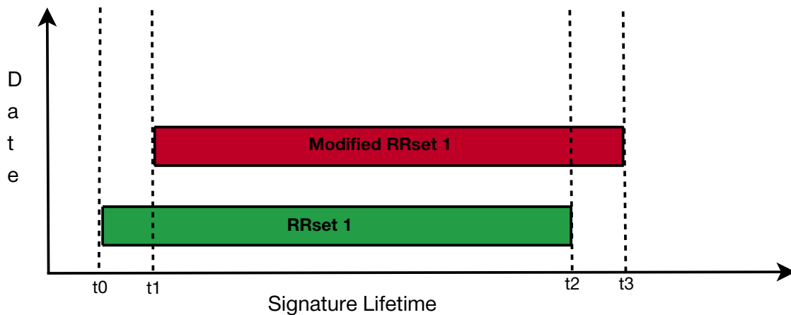
Figure 4.3 – If data changes, such as in Modified RRset 1, then the old RRset 1 will still be verified by the zone's keys (even though the data is no longer valid).
